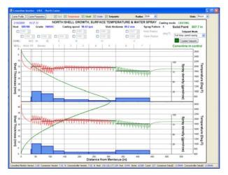
**Fig. 9.** Monitor interface displaying on both sides: the shell surface temperature profile, its corresponding setpoints, spray-water flow rates commanded and their setpoints, shell thickness profile prediction, and other information.
