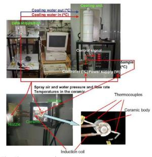
Fig. 19. New steady-state measurement apparatus
